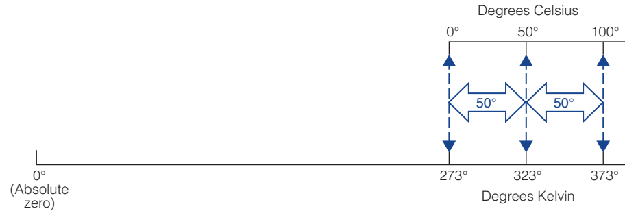
FIGURE 1.1 Three temperatures represented on the Celsius and Kelvin scales.
